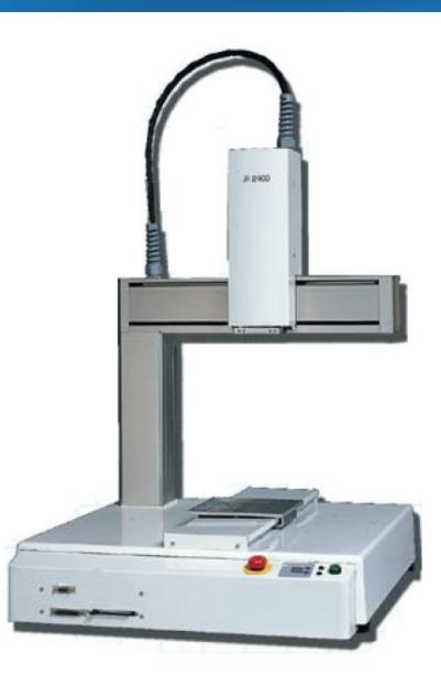
Even complex program patterns can be developed quickly using the simple point to point teach pendant. Dispense adhesive direct from syringes or optional metering valves and pressure pots. With fast indexing speeds, high accuracy and simple programming; robots are an ideal solution for most dispensing applications in a 400mm x 400mm work area. 3 or 4 axis versions available. Recommended optional light guard safety cages also available.
